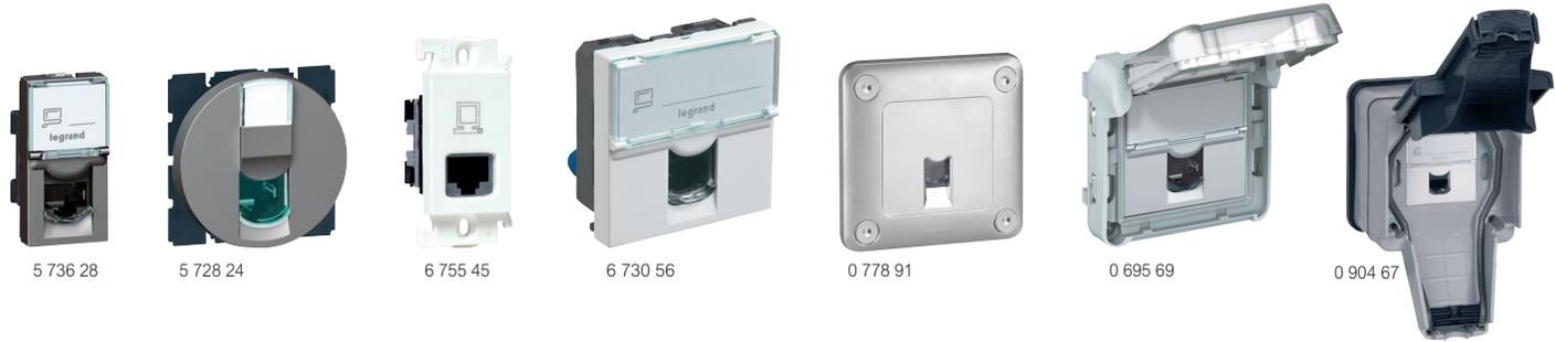
Sockets with LCS<sup>3</sup> quick-fixing crimp connector. Take AWG 22 single-core cables up to AWG 26 and AWG 24 multicore cables. Contacts marked with dual colour code and wiring schemes T 568 A and T 568 B. Conforming to standards ISO/IEC 11801 Ed. 2.0, EN 50173-1 and TIA/EIA 568
